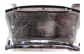
Complete the installation by removing excess material that would interfere with normal operation of any hinges or latching mechanisms.
